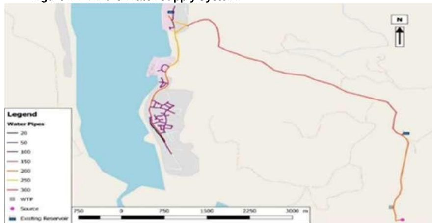
Figure 1--1: Noro Water Supply System
